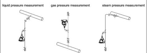
Figure 2. Examples of pressure transmitter installation
