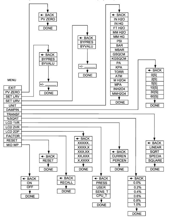
Figure 13. Local menu structure of transmitter
