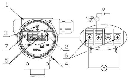
Figure 5. Electrical connection to transmitter
