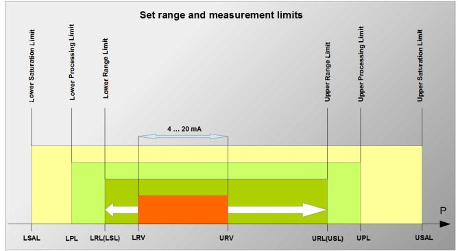
Figure 1. Set range and measurement limits
